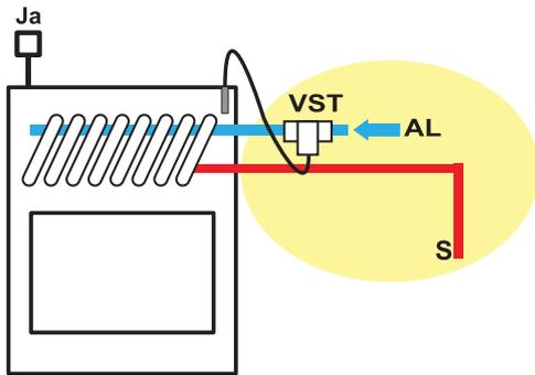
The thermal relief valve (TRV - provided by Edilkamin) must be connected to the cooling circuit (AL) with a minimum pressure of 1.5 bar.
