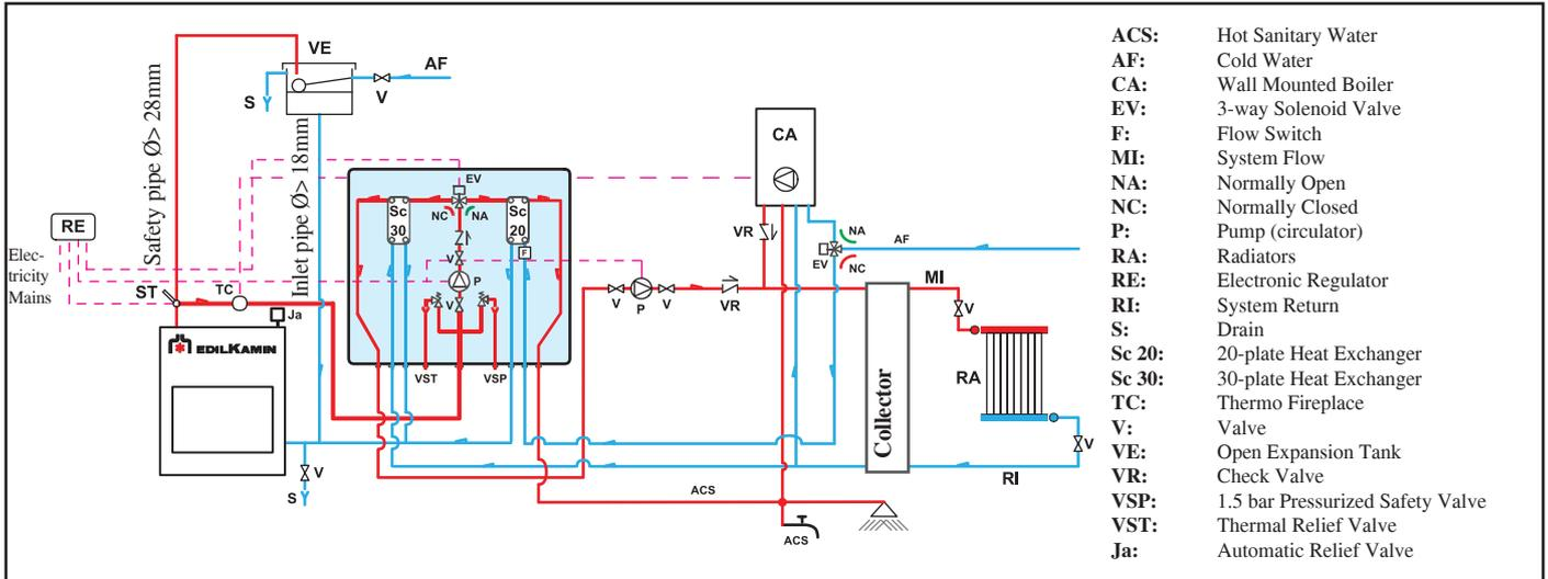
Kit 3 is designed to facilitate the work carried out by the installers. In fact, it consists of all the necessary components for the product to be properly installed.
