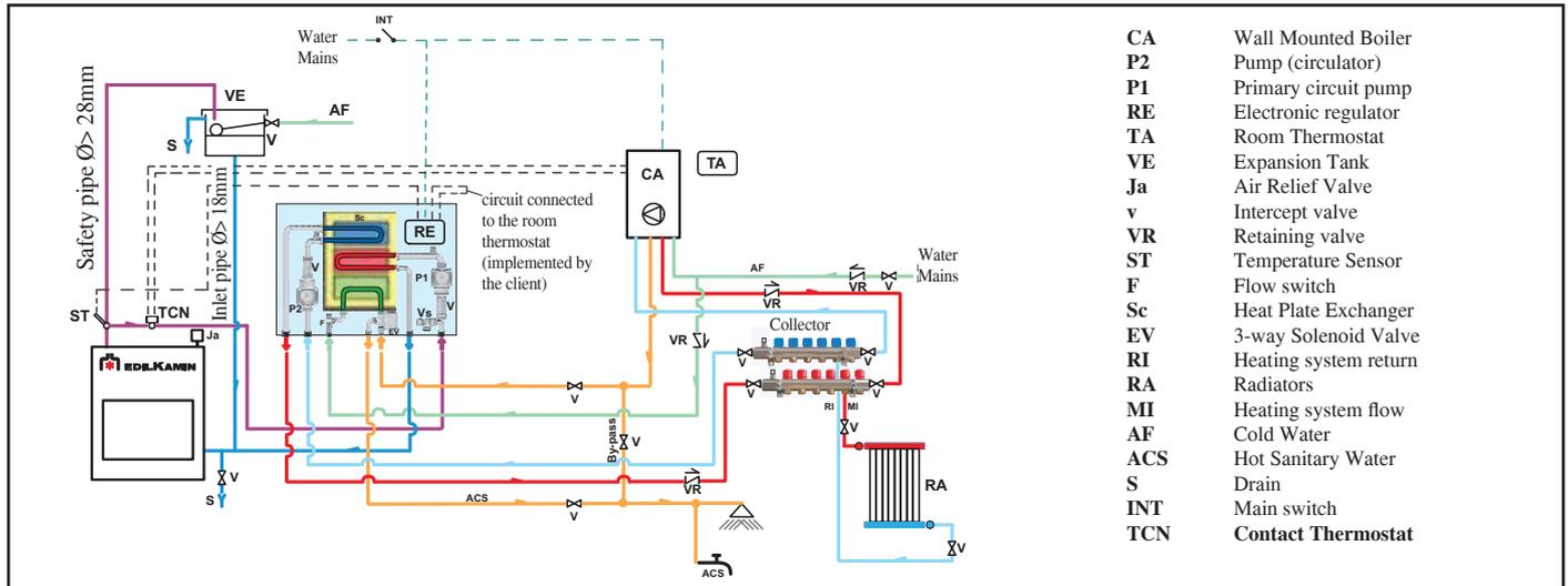
Kit N3BIS is designed to facilitate the work carried out by the installers. In fact, it consists of all the necessary components for the product to be properly installed.
